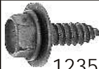
12351 (11505022) Black Polyseal Finish M6.3-1.81 x 20mm (#14 x 25/32") Hex Washer Head Sems® 17mm (11/16") Wshr O.D. 10mm Hex GM
