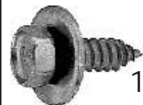
12351 (11505022) Black Polyseal Finish M6.3-1.81 x 20mm (#14 x 25/32") Hex Washer Head Sems® 17mm (11/16") Wshr O.D. 10mm Hex GM
